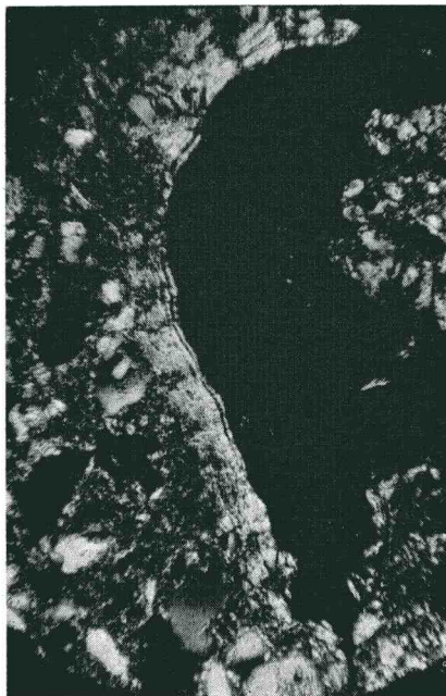
Fig. 3.—Clay skin (white banded area) enclosing a soil pore (black) as seen under a polarized light microscope.
