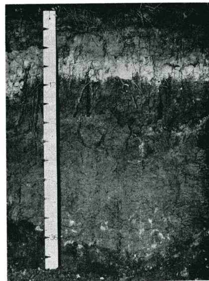
Fig. 2.—Gray Wooded soil (Typaltal) on a Manitoba lake clay. The A horizon is white (A 2 ) and overlies a clayey, somewhat blocky B. Below 24 in. is the C horizon.
