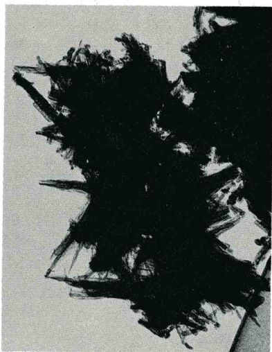
Cement paste after 16 hours, magnified 30,000 times. Inter-meshed fibrous crystals are tobermorite gel, the heart and strength of concrete.
