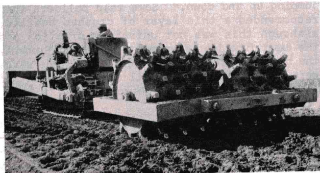
Soil compaction devices often copy the pre-eminent tread of animal feet. Above, a sheepsfoot roller. Right, a kind of bouncing bump-thumper used in Europe.
