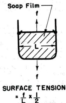
Obviously a pull,  $f$ , is required to keep the frame open due to surface tension of the soap film. Neglecting friction, the surface tension equals the force divided by the length of the wire and furthermore divided by two, because two soapy surfaces are at work, one on each side of the film.
