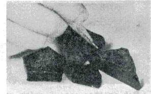
Natural rock asphalt from Kentucky--actually asphalt-impregnated sandstone.
