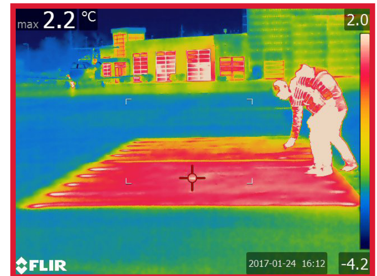
A thermal image of the heated airport pavements.
