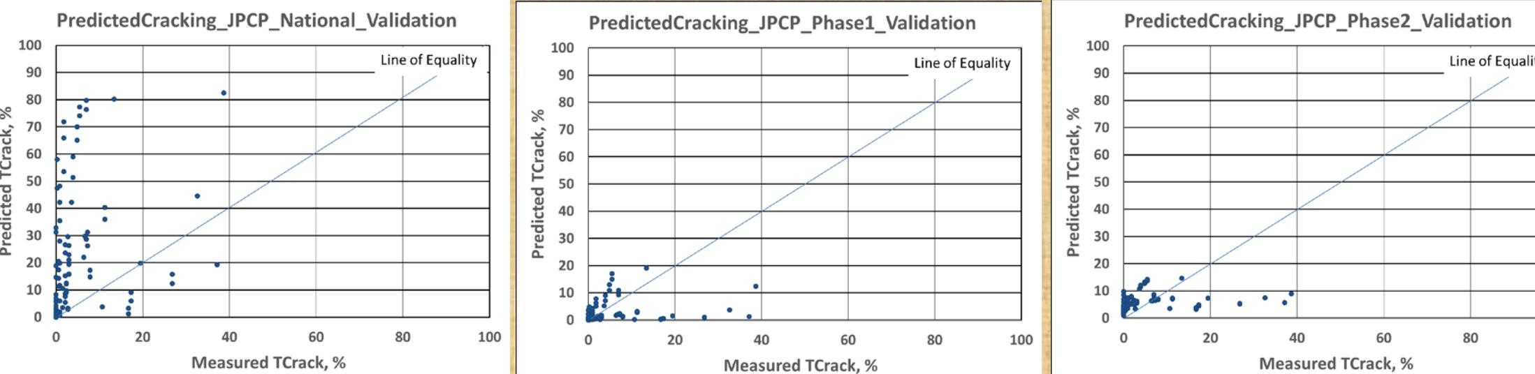
Overall summary of comparisons between measured and predicted JPCP transverse cracking
