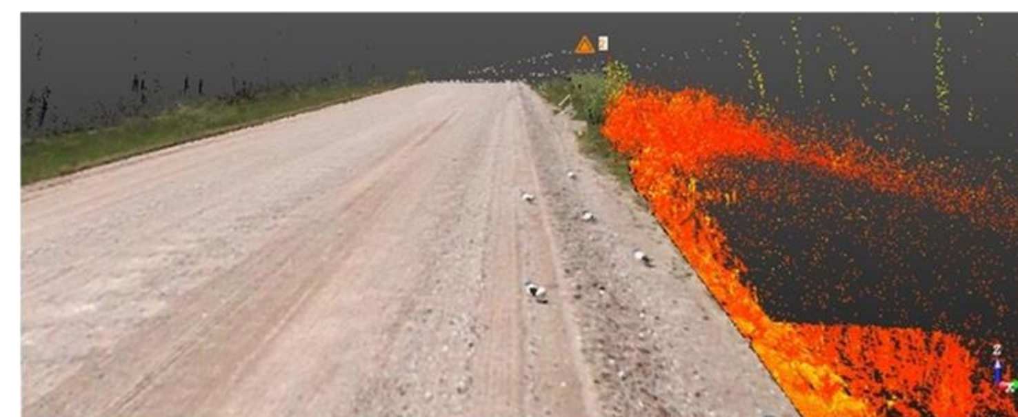
FIGURE 2 Registered point cloud for data acquired from two stations.
