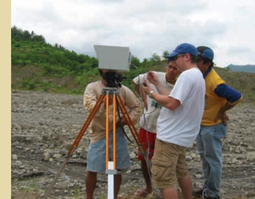
Researchers in the Philippines use terrestrial laser scanning equipment to gather data about the catastrophic landslide that occurred in St. Bernard in 2006.
