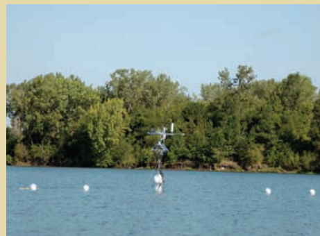
Researchers placed the above testing device in Ada Hayden Lake. It measures water temperature, wind speed, lake depth, and more.
